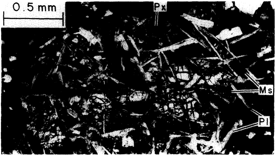
Fig. 2. ALHA 76005, Clast No. 1. Ophitic pyroxenes (Px) enclosing elongate laths of plagioclase (Pl), with scattered pools of dark mesostasis (Ms).
