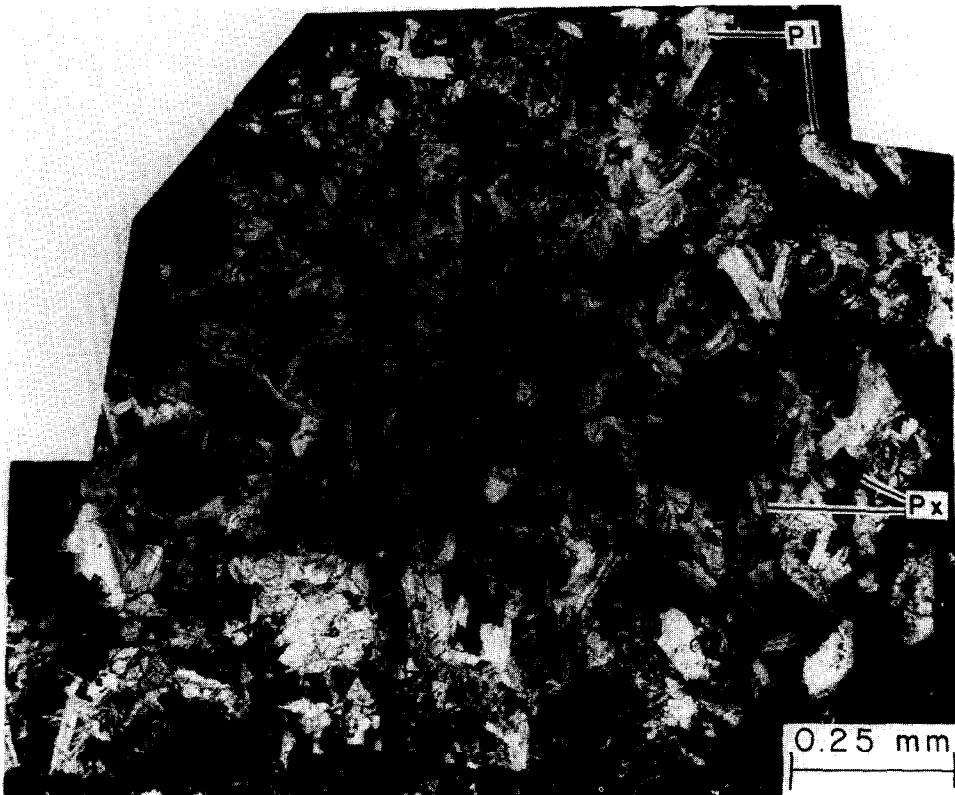
Fig. 5. ALHA 76005, Clast No. 2. Stubby plagioclase laths (light grey, Pl) with intergranular pyroxenes (dark grey, Px).
