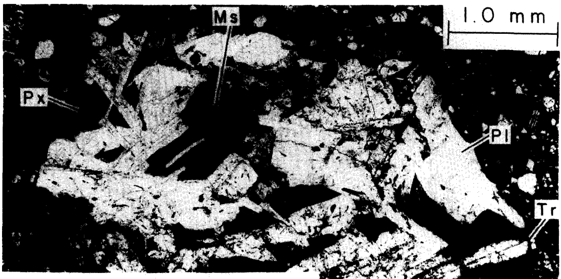
Fig. 7. ALHA 76005, Clast No. 6. Large, mostly euhedral plagioclase laths (white, Pl) and lesser tridymites (Tr, long white crystal), form a cumulate meshwork, the interstices of which are filled with anhedral pyroxenes (dark grey, Px), ilmenites (not visible in photo), and pools of dark mesostasis (Ms).
