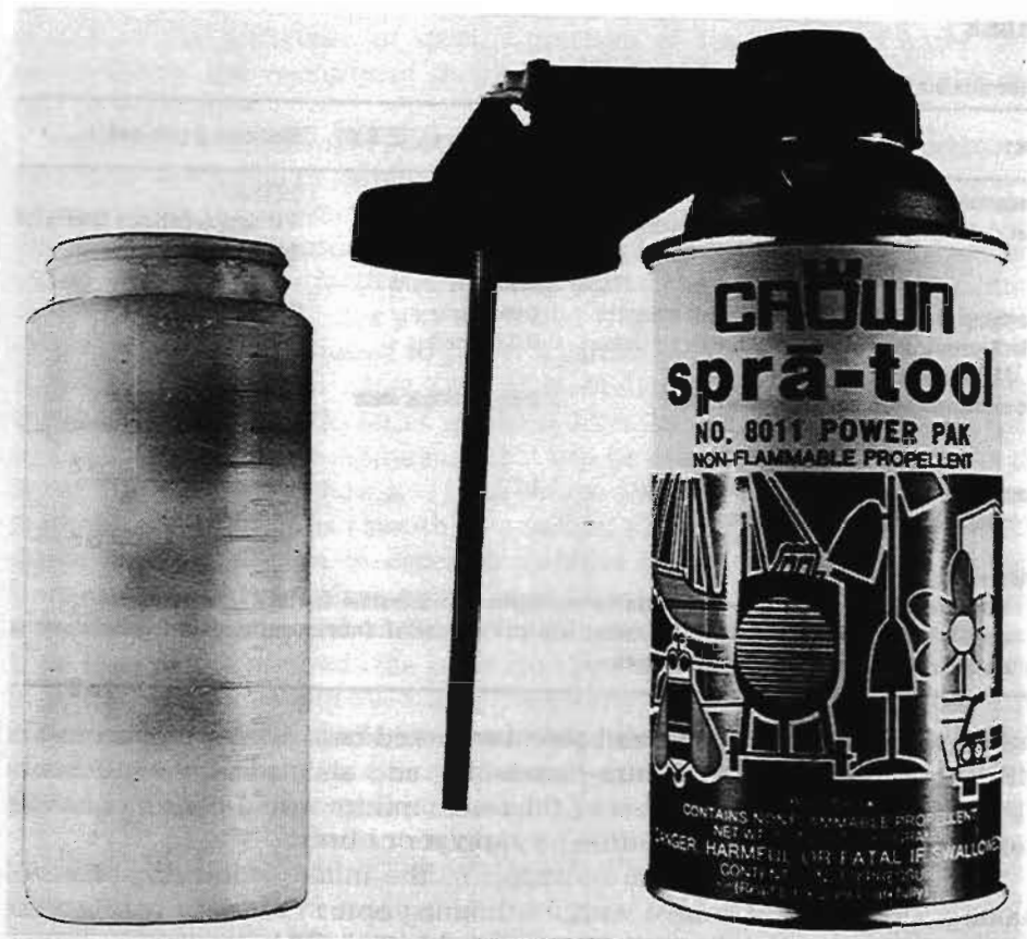
Fig. 1. Snap-on plastic spraying apparatus and can of propellant used to stabilize sediment surface with a mixture of polyester resin and catalyst thinned with alcohol.
