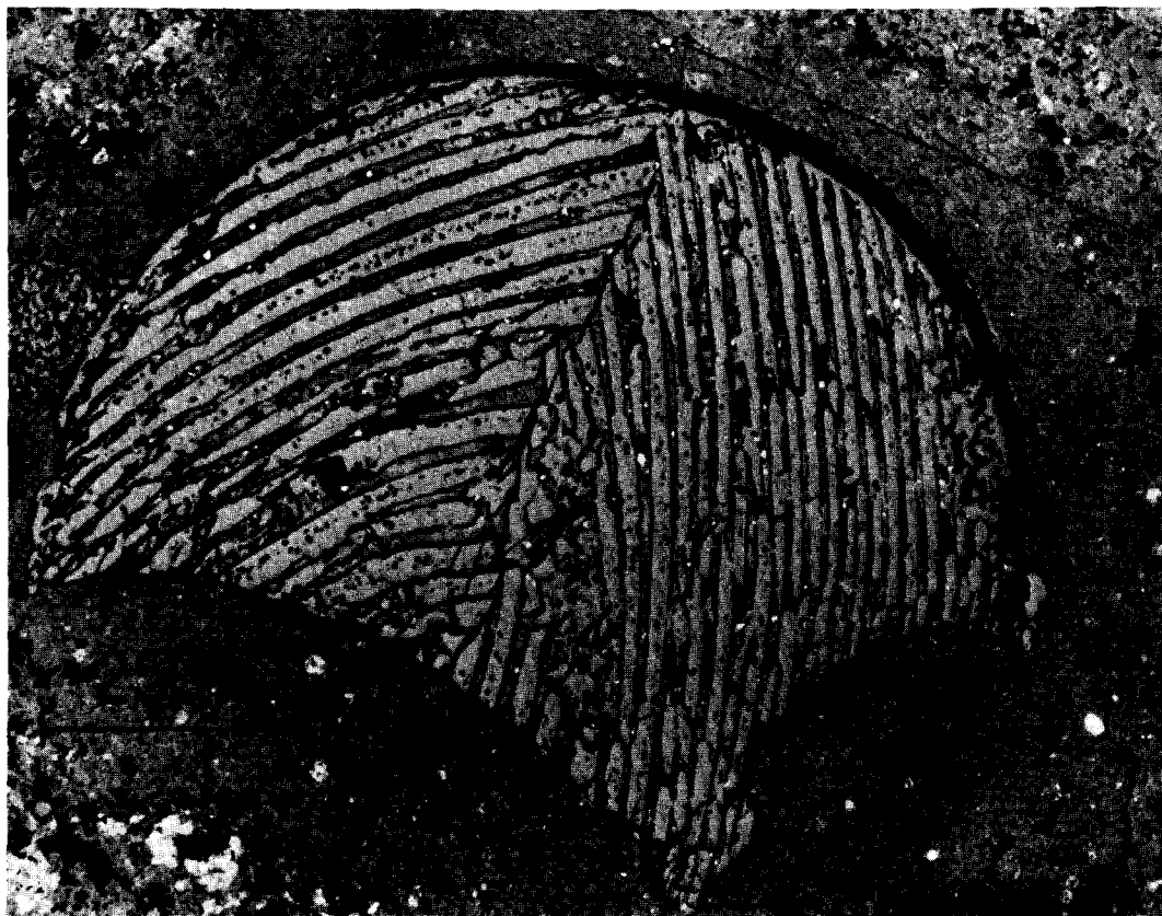
Fig. 9. Fragment of barred olivine chondrule in Murchison. The glass has been converted to green phyllosilicates. Apparently, this process did not facilitate breakage of the chondrule, since the fracture surface does not run along a phyllosilicate bar. Instead, it cuts across bars.
