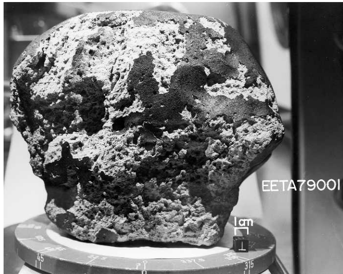
FIG. 2.—Martian meteorite Elephant Moraine, Antarctica (EET) A79001. This shergottite (basaltic) meteorite is a find, recovered long after it fell and after prolonged exposure to the Antarctic weathering environment. Weathering removed much of the black fusion crust, patches of which remain. This meteorite was the first SNC meteorite analyzed for inert and noble gases that matched those of Mars' atmosphere (Bogard and Johnson 1983) and was found to contain low-temperature aqueous alteration products, including clay mineraloids, carbonates, and gypsum, many of which are preserved in textures indicating their preterrestrial origin on Mars (Gooding 1986a, Gooding et al. 1988). See text for further details. NASA Johnson Space Center image S80-37480.
