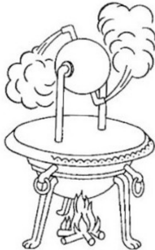
Impelling rotation by force of steam ejected through a nozzle
