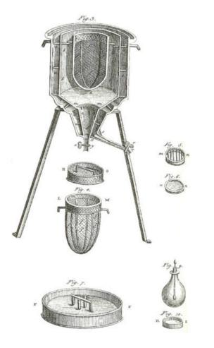
**Figure: Lavoisier's "ice calorimeter".** The fuel to be burnt goes in the dome-shaped chamber at the center, and ice is placed in the inner and outer jackets that surround it. When the fuel is burnt, heat is transferred to the ice in the inner jacket and melts it. Water from that melting ice drips out of the device and is collected below and weighed at the end of the experiment. The outer jacket serves just to insulate the inner jacket from the warm surrounding environment.
