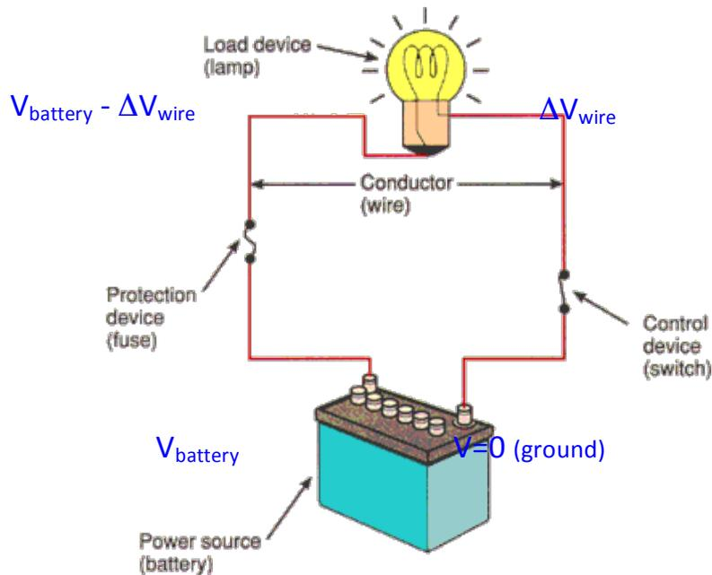
*Example of voltage drops in a simple electrical system. Blue labels show the voltage at different locations. This diagram assumes that the outgoing and return wires have the resistance  $R_{wire}$  and so each experience a voltage drop  $\Delta V_{wire}$ .*
