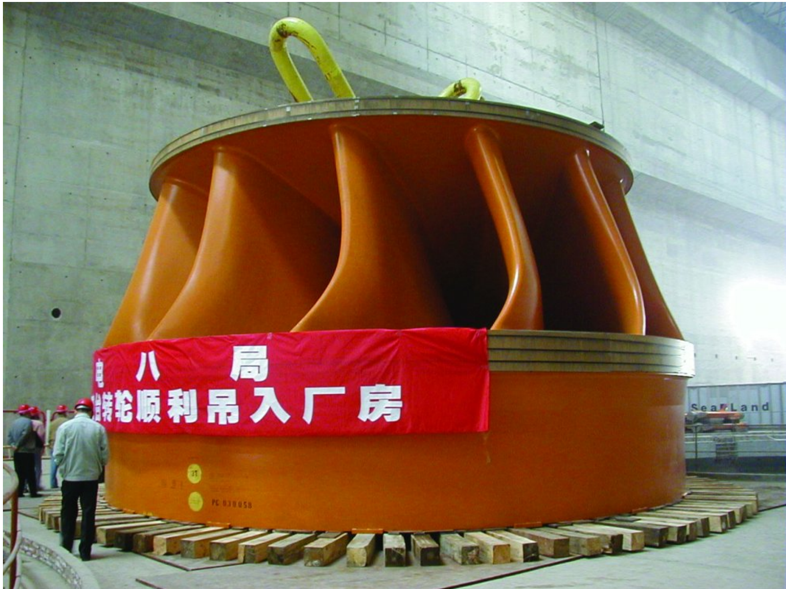
Francis turbine runner from Three Gorges Dam project, China (900 MW)
