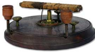
Figure 2: Ritchie motor from 1830's ( image from website cited above )
