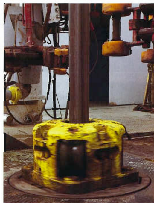
The main hoist on the Marlow rig (above) supports the drill string and regulates downward force. The black hose supplies drilling mud, which is pumped down the bore of the pipe. The rotary table (below) turns the drill string, transmitting twisting force to a special length of drill pipe called the kelly.
