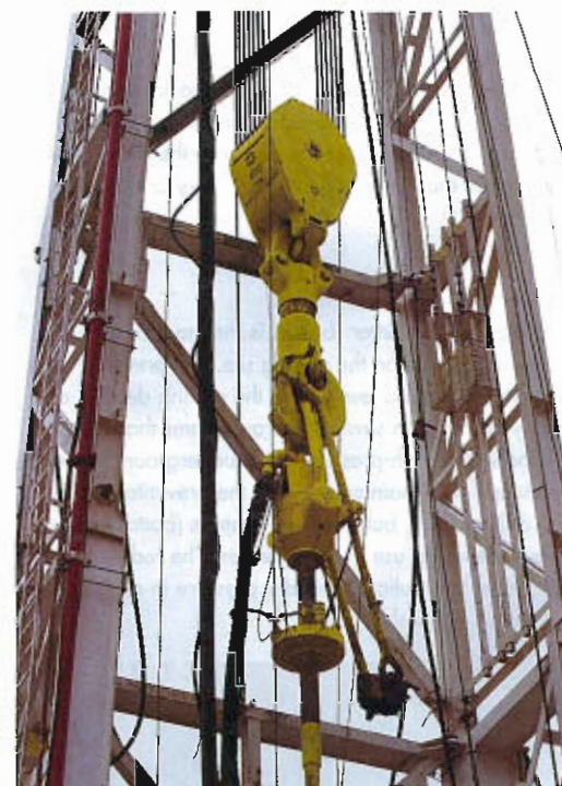
The main hoist on the Marlow rig (above) supports the drill string and regulates downward force. The black hose supplies drilling mud, which is pumped down the bore of the pipe. The rotary table (below) turns the drill string, transmitting twisting force to a special length of drill pipe called the kelly.
