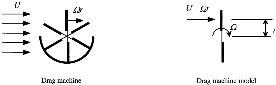
Figure 3.16 Simple drag machine and model; U , velocity of the undisturbed airflow; \Omega , angular velocity of wind turbine rotor; r , radius
