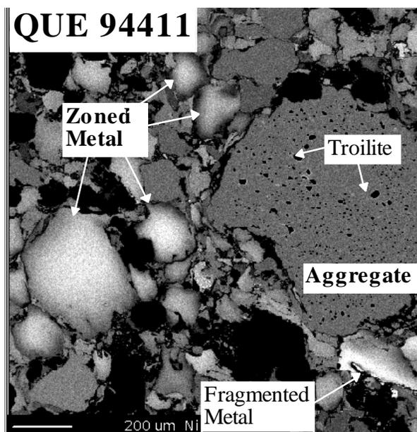
Fig. Ni X-ray map of the QUE 94411 CB chondrite. Brighter areas have higher Ni. Darkest areas are non-metal. Shown are zoned metal grains and a large metal aggregate with troilite blebs.
