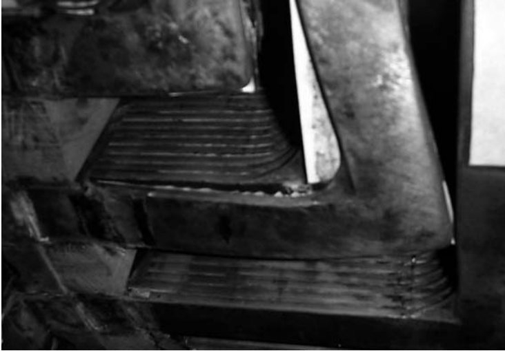
Fig. 4.17 Rotor field end-winding of a 90 MVA, 3600 rpm, hydrogen-cooled generator. The top turn of one coil has shifted during operation all the way across the gap separating it from the neighboring coil, resulting in a severe shorted-turns condition. This is the result of ratcheting during cycling and insufficient blocking.
