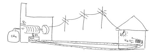
**Above:** Cogeneration type #1: making just enough electricity to meet your electrical needs (and burning extra fuel in a furnace if you need more heat.)
