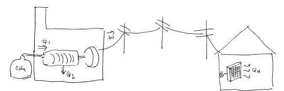
**Above:** heating via chemical  $\rightarrow$  heat  $\rightarrow$  electricity  $\rightarrow$  heat **Below:** heating via chemical  $\rightarrow$  heat
