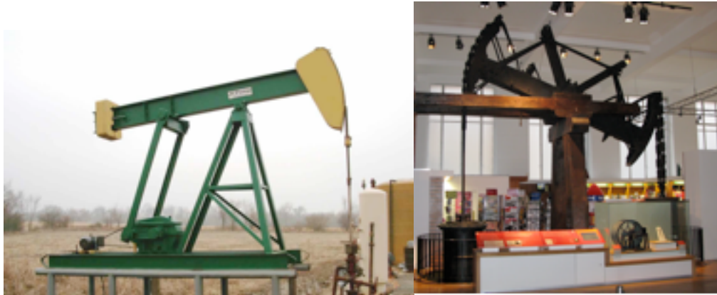
L. Pumpjack, R. Watt’s “Old Bess” engine, both used for pumping liquids
