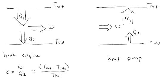
The best heat engine would be a purely reversible one – that is, it would suffer no frictional or other losses. In this case the values of all the heat flows are identical no matter which direction the engine is run in.
