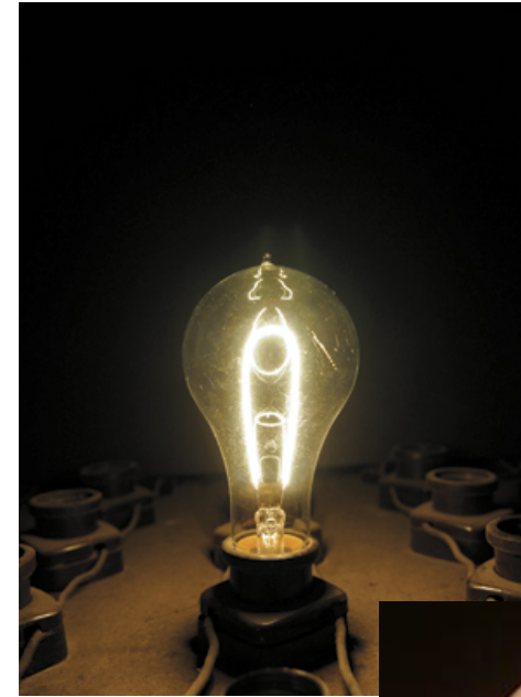
Replica of Edison's 1890 carbon filament bulb ( J. & L. Casey )
