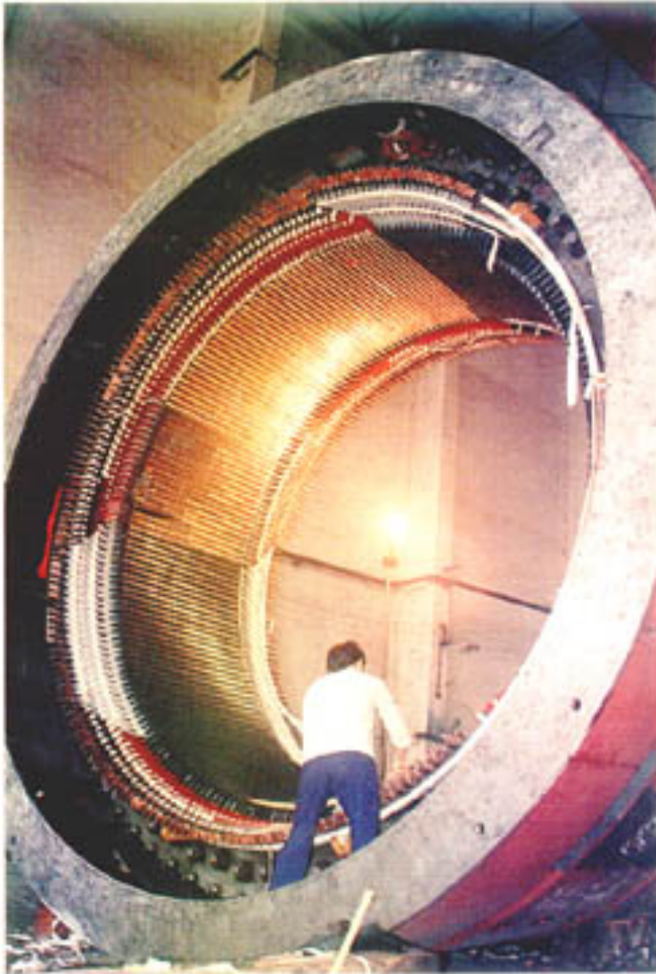
Stator, 3-phase generator, Welluck Co., China, 12.5 MW, 2010
