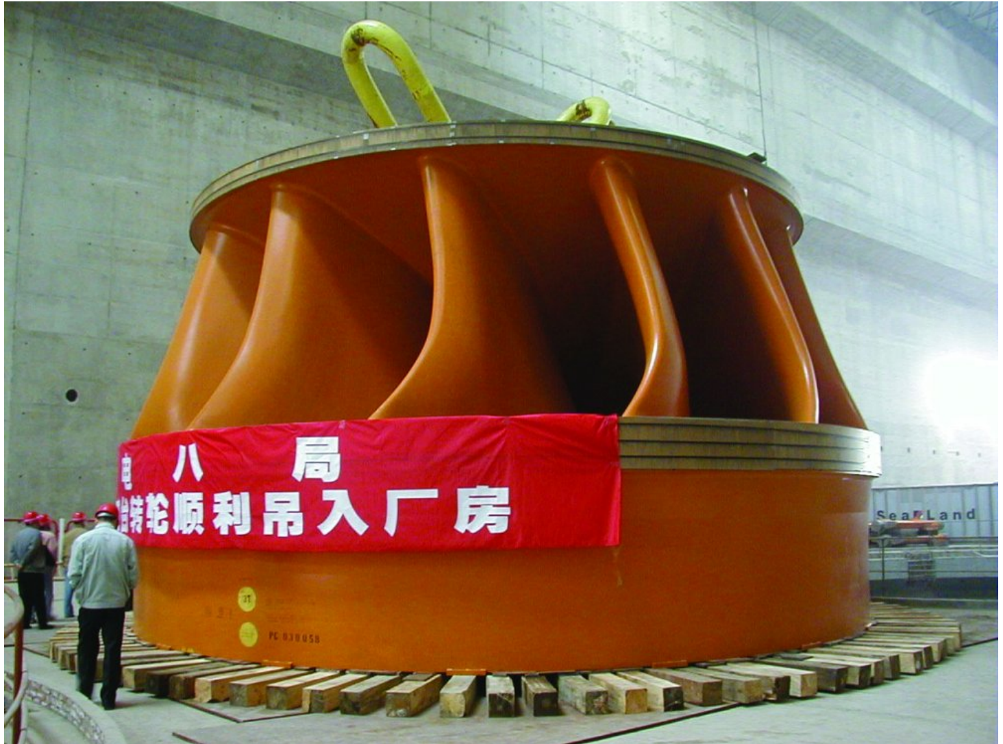
Francis turbine runner from Three Gorges Dam project, China (700 MW)
