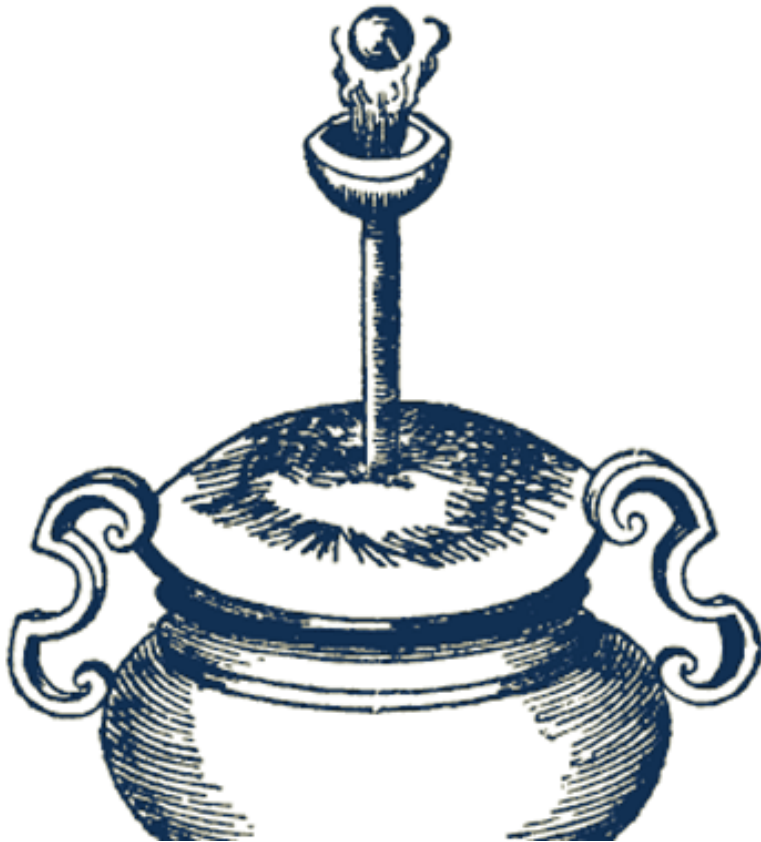
“lebes”: demonstration of lifting power of steam
