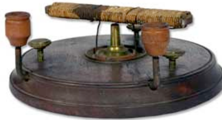
Rotating electromagnet, Wm. Ritchie, 1833
