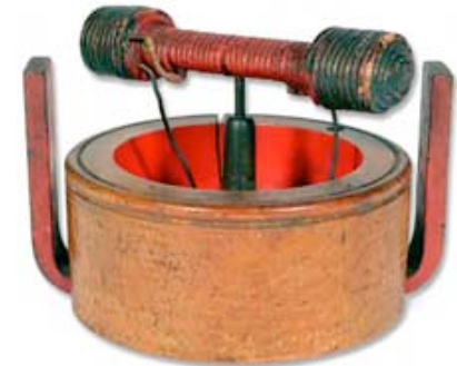
Rotating electromagnet, Wm. Sturgeon, 1838
