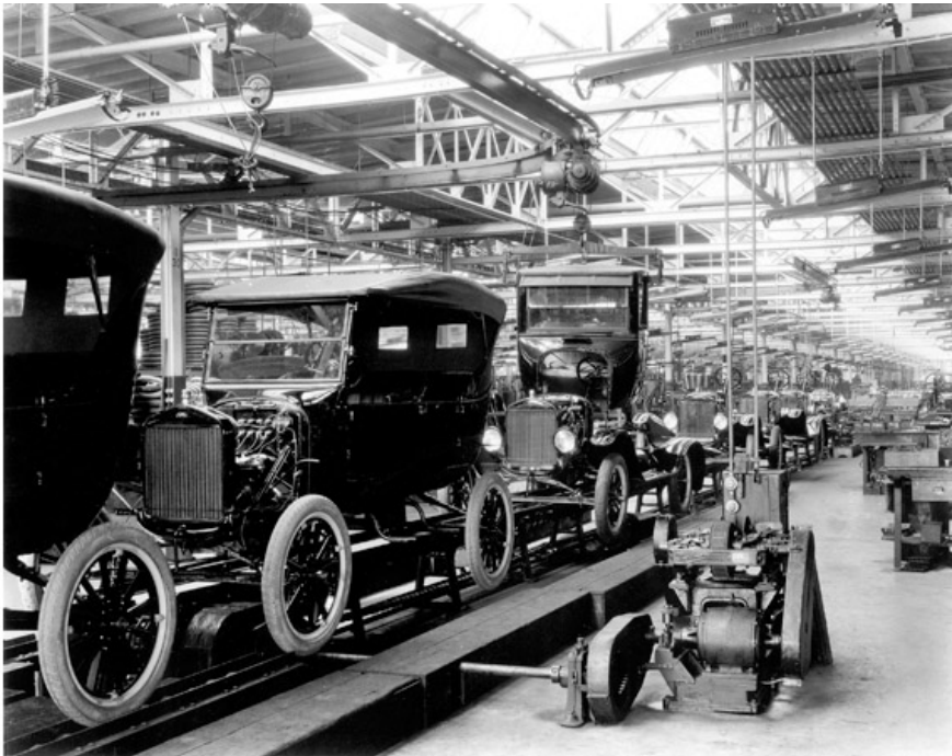
Ford Model T assembly line, 1924.
